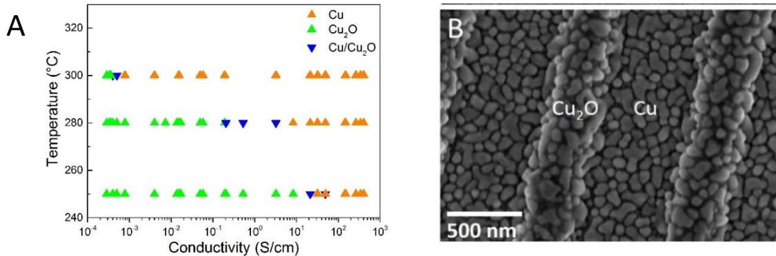
Figure 1: a) diagram showing the deposited material as a function of substrate conductivity. b) SEM image of a Cu and Cu<sub>2</sub>O simultaneous deposition surface with alternating areas of low and high electronic conductivity.
